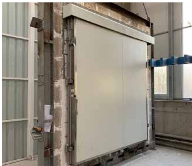
Testing according to CE EN 1634-1 and UL 10C:2021 Fire Protection Standard
