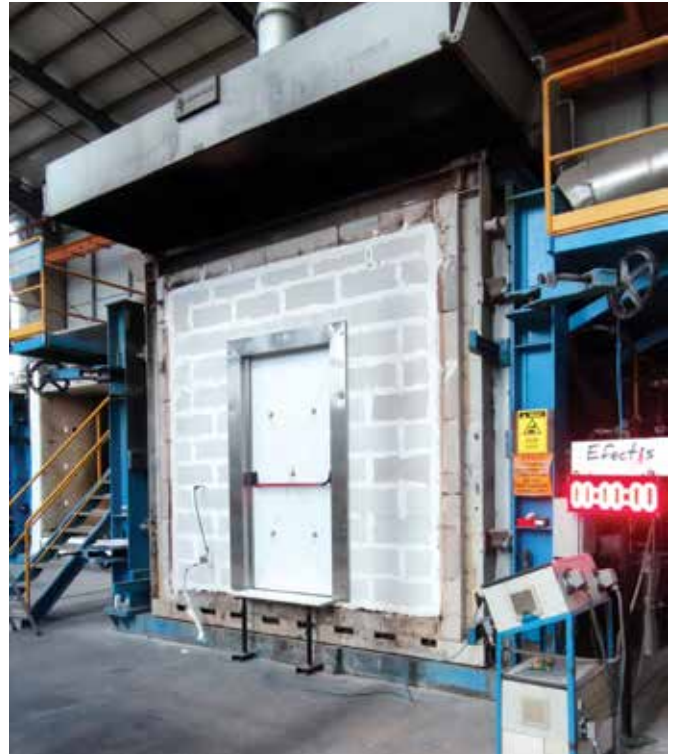
Testing according to CE EN 1634-1 and UL 10B: 2021 Fire Protection Standard
